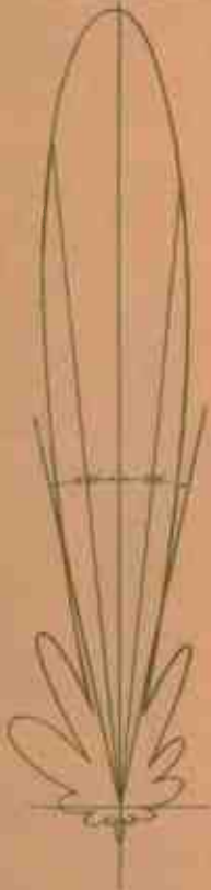
THE FIELD STRENGTH CURVE. This polar curve gives some idea of the narrow path followed by the signals from the radio lighthouse.
