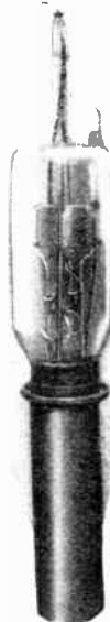
One of the high-power water-cooled vacuum tubes is shown at the left. The plate of the tube is the metal cylinder at the bottom, from which the heat is dissipated by the cooling water.
