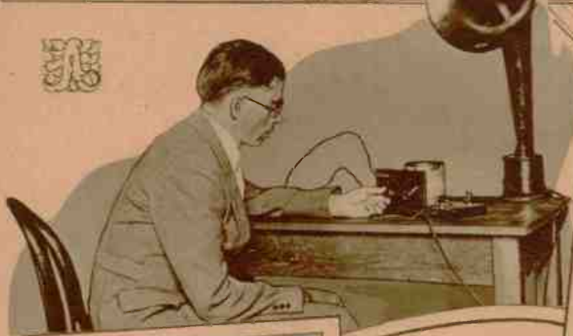
CRYSTAL SET OPERATES LOUD SPEAKER. In the Radio Laboratory of the Bureau of Standards in Washington, Morris S. Strick has succeeded in obtaining signals from a loud speaker using a crystal detector alone. He states that a big antenna and a good crystal are necessary. © Harris & Ewing.
