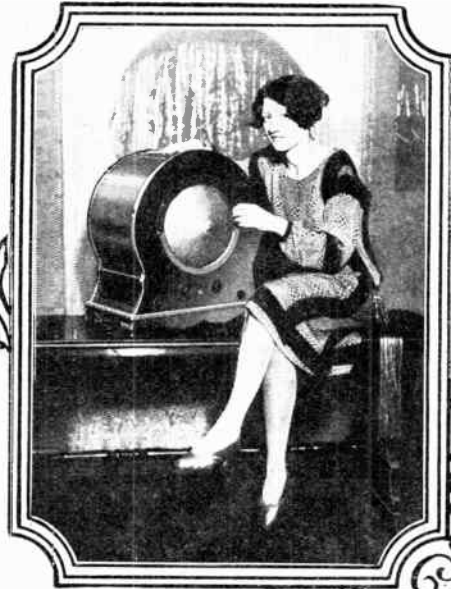
A UNIQUE RADIO RECEIVER. The cone loud speaker in this set acts also as a dial for tuning as well as performing its usual duty. © Fotograms.
