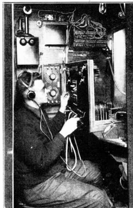
A monitor is in charge of the signals as they go from the land line to the radio link in the transatlantic chain.
