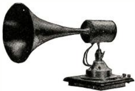
One of the Loudspeakers Embodying a New Principle of Construction. The Mechanism is in the Cylinder, Upon Which is Mounted the Horn, and May Be Adapted to Any Type of Sound Box
