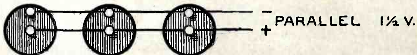
Fig. 1. Three Dry Cells Connected in Parallel Give 1 1/2 Volts for W D 11 or W D 12 Vacuum Tubes
