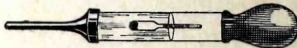
Fig. 3. A Hydrometer Used for Testing the Specific Gravity of the Electrolyte in a Storage Battery
