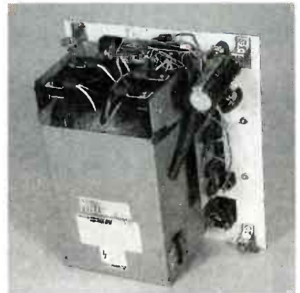
FIG. 3—THE PROTOTYPE INVERTER. The author used a car cigarette lighter plug on the end of the power-input lead and an AC outlet for plugging appliances into.
