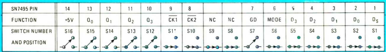
FIG. 6—SWITCH SETUP for testing the 7495 4-bit shift register.
