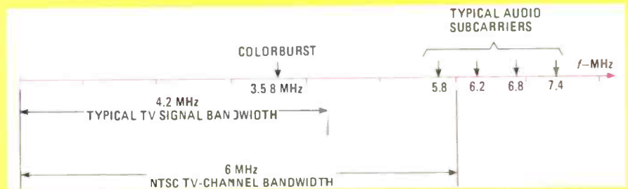
FIG. 1—THE TYPICAL SUBCARRIER FREQUENCIES used for audio transmissions are 5.8, 6.2, 6.8, and 7.4 MHz.
