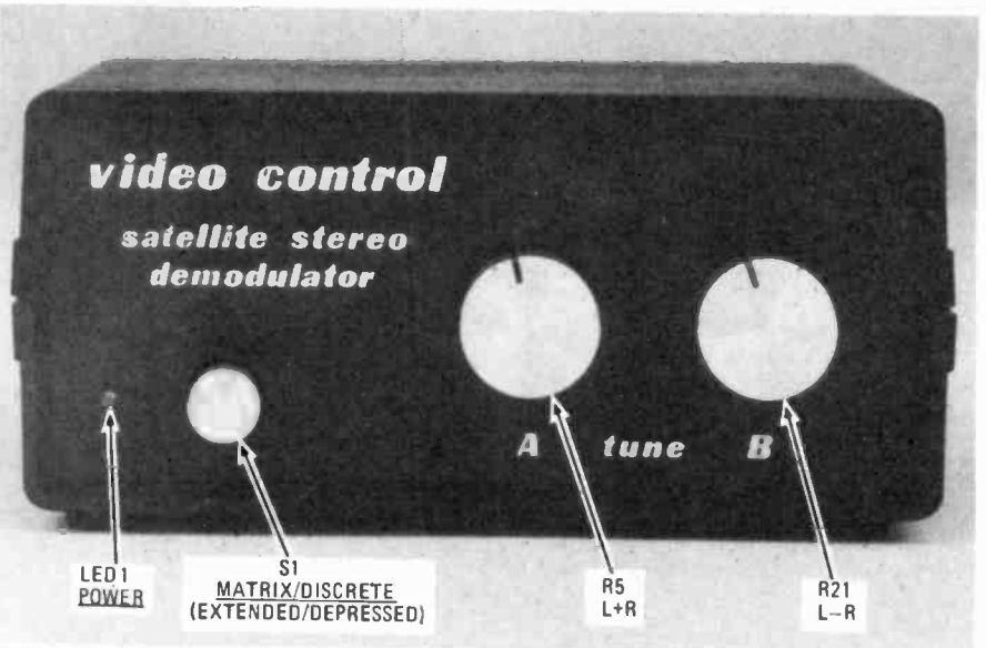
FIG. 9—FRONT-PANEL CONTROLS. To make the unit easier to use, you might want to mark the settings for your favorite transponders around the tuning controls.
