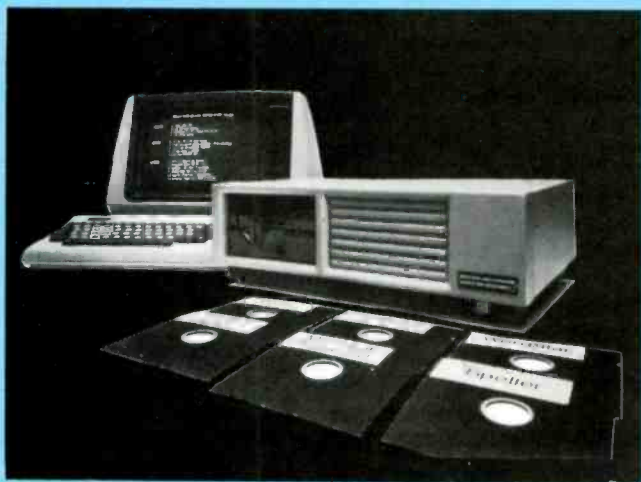
MORROW DESIGNS MICRO DECISION MD1 is a CP/M machine that includes bundled software.
