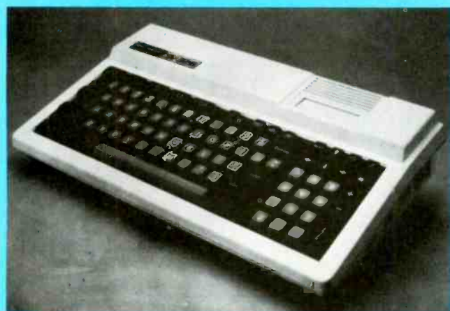
SPECTRAVIDEO'S SV-328 uses a Z80A microprocessor.
