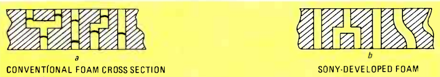
FIG. 8—NEW FOAM MATERIAL (b) developed for the MDR-series headphone earpads has no walls across the sound path, improving sound quality.
