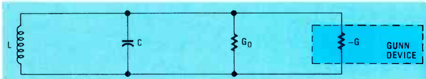
FIG. 6—GUNN DEVICE is shown as a negative conductance placed in parallel with an L-C tank circuit. The circuit will oscillate if -G is much greater than G_0 .
