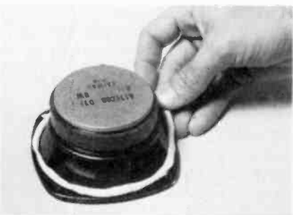
FIG. 4—CAULKING COMPOUND is used to give air-tight seal when speakers are mounted.
