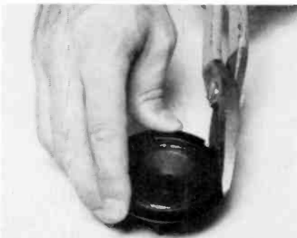
FIG. 3—TREBLE DRIVER'S FRAME is trimmed using metal-cutting shears.
