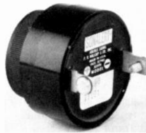
FIG. 1—THE PIEZOELECTRIC SOUNDER is a low-current device that produces an almost pure tone. This is a Sonalert, made by the Mallory Components Group of Emhart Corp.
