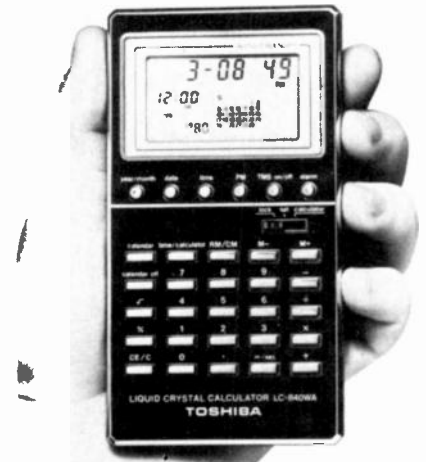
THE TOSHIBA LC-840WA CALCULATOR can show, at one time, the calendar for the month, with present date flashing, the time down to the second, and the time for which the alarm has been set.
