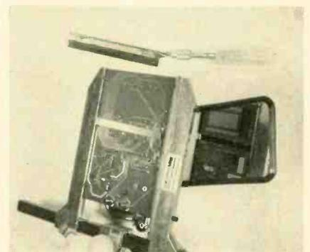
**FIG. 4—**STRAIGHT CUTS in PC board is made with modeling saw.
