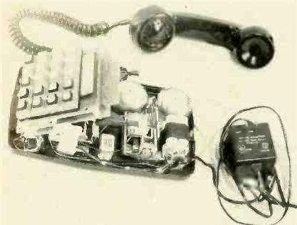
INSIDE VIEW of the Superphone 7710. The buzzer is used as an alarm signal. Rechargeable batteries retain memory if the power fails.
