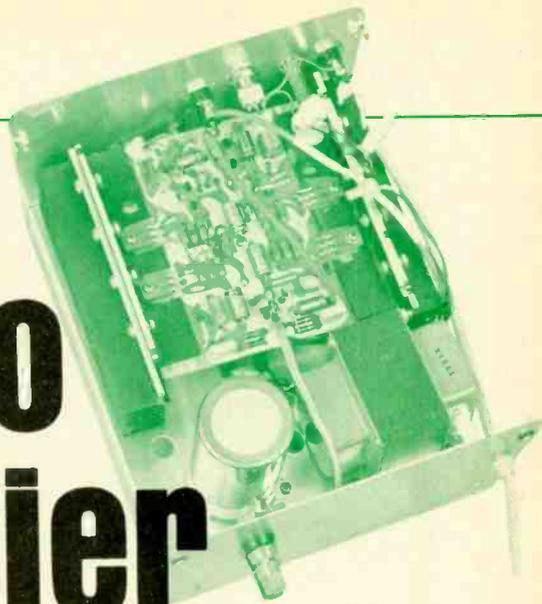
*Bridge-type power output configuration lets you use inexpensive "plastic" transistors and a simpler power supply to provide a wide frequency response and a signal-to-noise ratio of 100 dB.*
