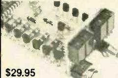
0106 Displays either hours and minutes, month and day, or seconds. Requires only 2 mA of current while ignition is off. Also operates on 9V battery. Mounts easily in compact two-inch enclosure (Not included)
