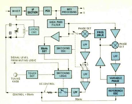
BLOCK DIAGRAM OF DISTORTION-DETECTION LOOP (DDL)
