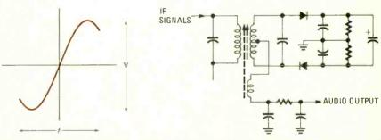
FIG. 1—CONVENTIONAL DISCRIMINATOR has a nonlinear S-curve characteristic to convert FM signals into AM signals.
