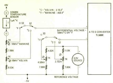
FIG. 4—BASIC DIAGRAM of circuit used for temperature measurement. The temperature sensor is a current source; passing 1  $\mu$ A-per-degree Kelvin. Readout is in °C and °F.
