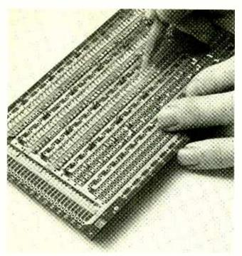
UNIVERSAL PC BOARD and wiring pen manufactured by Vero Electronics, Inc.
