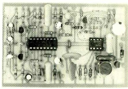
TOP VIEW OF THE PC BOARD shows the locations of most of the components. Parts not shown include the bar-graph display and power supply.
