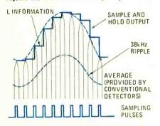
SAMPLE-AND-HOLD DETECTOR FOLLOWS 38kHz ENVELOPE PEAKS AND REQUIRES LESS FILTERING.
