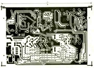
FIG. 6—PATTERN for the under side of the main PC board shown half-size. The pushbutton range and function switches are on this side.
