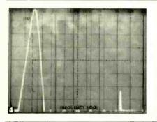
With our spectrum analyzer set to its higher sensitivity mode (2 dB of amplitude per-vertical-division), we first examined the output with the expansion control set for 1.0 (no expansion). Figure 3 shows the response from 20 Hz to 20 kHz. Note that the 60-Hz component at the output is some 7-dB greater than the 7-kHz contribution to the overall signal.
