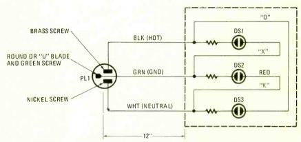
FIGURE 1—OUTLET POLARITY CHECKER. A simple and sure way of knowing if the outlet that you are about to plug into is functioning properly.
