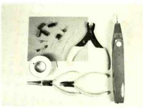
FIG. 2—TOOLS AND MATERIALS required for the cut/strip/hook wiring method.
