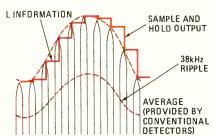
SAMPLE-AND-HOLD STEREO DECODING circuit is just one of the new circuits manufacturers are using for increased FM tuner performance. To find out what the circuits look like and how they work, turn to page 57.
