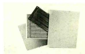
FIG. 1—PERFORATED BOARDS are used with the cut/strip/hook and wire-wrap wiring methods. Also shown is a universal-type printed-circuit board.
