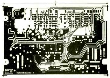
FIG. 5—FOIL PATTERN for Side 1, the top surface of the main board. Pattern is approximately one-half size. Enlarge to 71/4 inches across.
