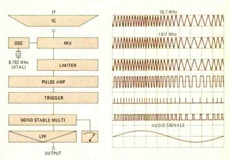
BLOCK DIAGRAM OF PULSE COUNT DETECTOR
