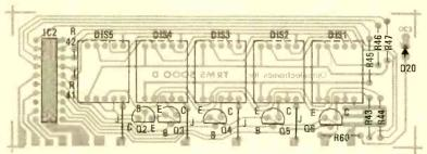
FIG. 12—DISPLAY BOARD parts placement. The IC is the display segment driver. The transistors are used in digit multiplexing.
