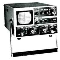
X-Y operation. Vertical modes include Channel-A only, Channel-B only, A & B, A + B and A - B. Timebase automatically switches between chopped or alternate sweeps. Unit operates on 117 VAC, 234 VAC, 12 VDC; an optional rechargeable battery pack is also available for incase mounting. Other options include a carrying case and demodulator probes. Provided with
