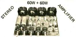
OCL pre amp. & power stereo amp. with bass, middle, treble 3-way tone control. Fully assembled and tested, ready to work. Total harmonic distortion less than 0.5% at full power. Output maximum is 60 watts per channel at 8  $\Omega$  . Power : 36  $\vee$  AC or DC. Complete unit . Power supply is 24
