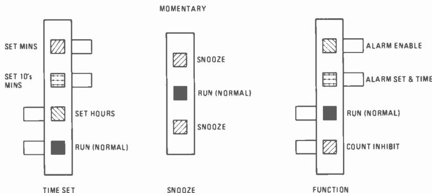
FIG. 8—SWITCH FUNCTIONS of the three slide switches.
