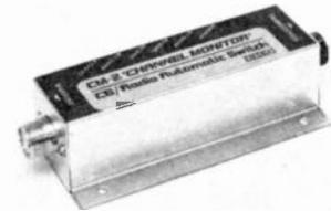
operation. The CM-2 is sensitive to both audio and RF so it will also silence when you transmit.
