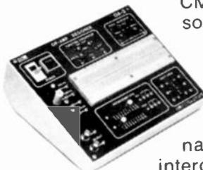
Powerful design tool for linear work and CMOS digital circuitry. SK-10 socket. Heavy current capacities on all three power supplies [+/- 15V & +5V DC]. Sensitive null detector and a full function generator with external frequency adjustment. All interconnections are solderless. \$95.00 in kit form.
