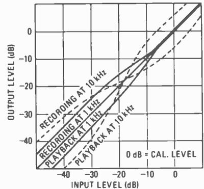
FIG. 8—INPUT/OUTPUT characteristics of the Super-ANRS circuit.
