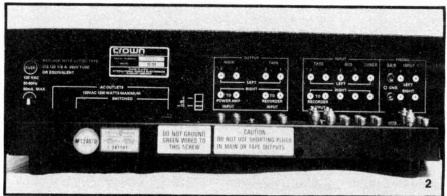
vertical surface for legibility. Near the pairs of PHONO inputs are screwdriver adjustment controls that permit you to vary the gain of the phono preamp section over a 20-dB range, with maximum sensitivity being 0.7 mV for rated output. In all of our subsequent tests, these controls were set to provide rated output (2.5 volts) from the main outputs with a phono input level of 2.5 mV. A slide-switch changes the gain by a fixed 10 dB.
