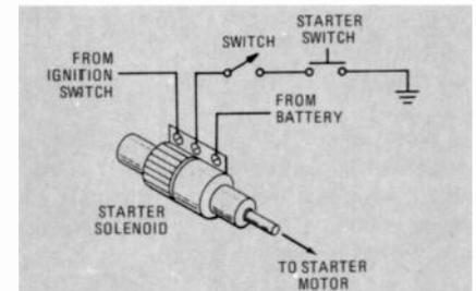
FIG. 3—STARTER IMMOBILIZER operates by opening starter-motor circuit.
