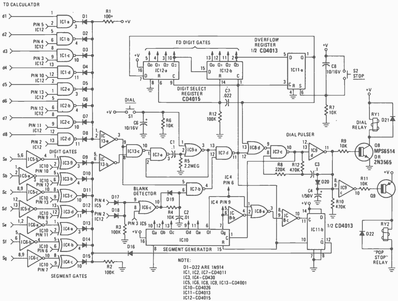
FIG. 1—THE TELEPHONE DIAL CONVERTER. Connections marked d1, #1, etc., are connections to the calculator (see Fig. 2).
