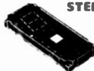
0.27" 7 segment LED, Latch and Driver built in one chip
