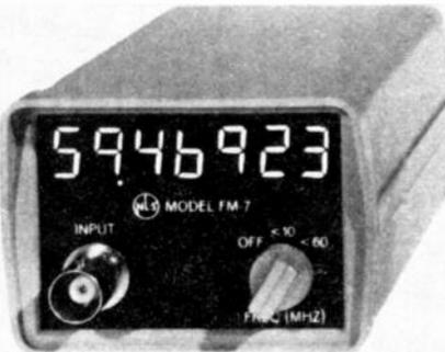
Resolution is 1-Hz below 10 MHz and 10-Hz from 10 MHz to 60 MHz. The internal timebase has an aging rate of less than 10 PPM from 0°C to +40°C. The unit operates on self-contained
