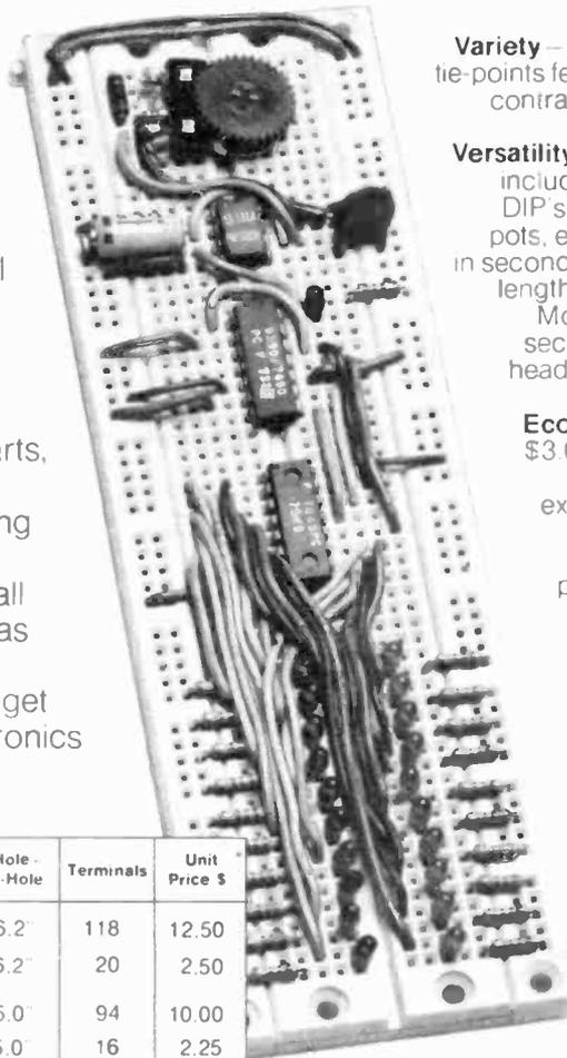
**Variety** — 10 models from 70 to 590 solderless tie-points feature snap/lock design to expand or contract your breadboard to fit every circuit and budget requirement.
