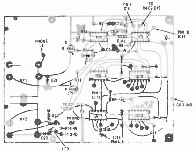
FIG. 6—COMPONENT LAYOUT of Board B.
