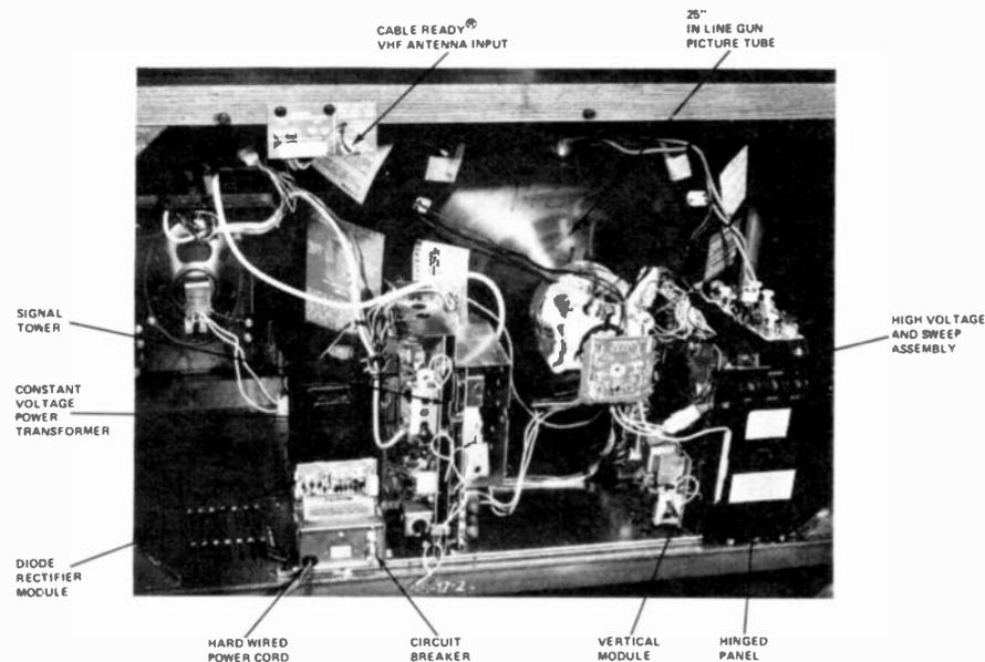
REAR VIEW of G-E's new television receiver containing the VIR module.
