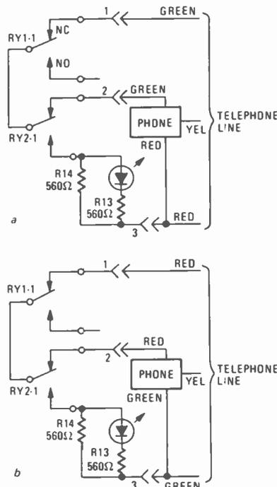
FIG. 7—TELEPHONE CONNECTIONS. Use the connection (a or b) that makes terminal 1 positive, or the one that causes dialing indicator to light when dialing.
