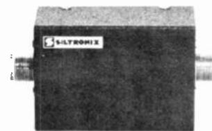
TVI-producing harmonics that are produced by many radios. The cutoff frequency is 30 MHz. Impedance is 50 ohms. Maximum SWR is less than 1.2:1 at 27 MHz.—Siltronix
