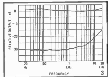
STR-130). Nominal output measured at 1 kHz was 3.0 millivolts for a stylus velocity of 3.54 cm-per-second. This corresponds quite closely to the 4.0 mV claimed by AKG for a velocity of 5.0 cm-per-second.
