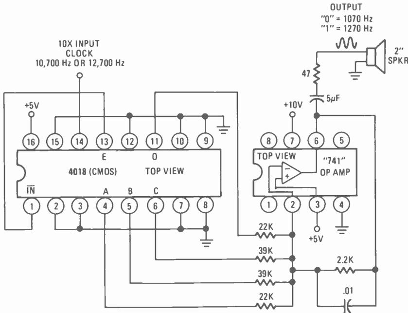
resistor value has been rounded off to a stock 1 percent value. Actually, 5 percent resistors are more than adequate for practically all sinewave generators, particularly for those of ten stages or less.
