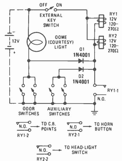
FIG. 7—MICROSWITCH-ACTIVATED alarm/immobilizer designed to operate on vehicles with +V ground electrical systems.
