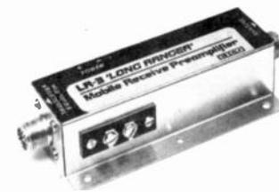
the receiver input, the LR-3 boosts received signals without in any way degrading the transmitted signal. A "sniffer" circuit senses the presence of transmitted RF signals and automatically causes the transmitted signal to bypass the receive preamplifier and be fed directly to the antenna.
