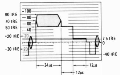
THE VIR SIGNAL makes color TV pictures perfect. It's tucked away on line 19 between two horizontal sync pulses. See how it works on page 83.
