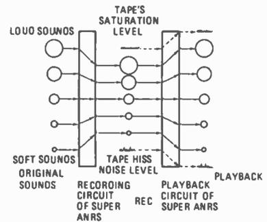
FIG. 7—COMPRESSION/EXPANSION characteristic of Super-ANRS circuit. The size of the circles are proportional to the signal levels.
