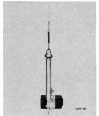
inches of chrome-plated stainless-steel telescoping mast with 18 feet of coaxial cable. Retracts into the fender well to within 3 inches of the mounting surface. The preferred location is in the left rear fender. Center loaded. SWR 1.3:1. \$64.95.—Tenna Corp.
