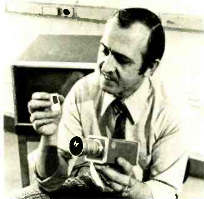
THE CHARGE-COUPLED IMAGE SENSOR is a single chip of silicon covered with an array of more than 235,000 electrodes.
