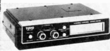
COMPATIBLE CARTRIDGE deck handles 4-channel and 2-channel stereo tapes. It's Toyo Qadio model CS-721.
