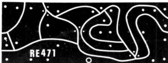
FULL-SIZE CIRCUIT BOARD pattern for the low-fuel alarm. Follow it exactly.
