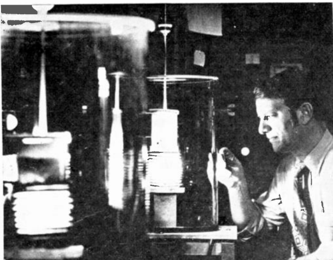
SPACE DAM FOR INTEL SAT IV COMMUNICATIONS SATELLITE. The multiplexer assembly (resembling spokes in a wheel) acts as a dam to separate the river of received signals into controlled streams of signal frequencies for this communications satellite built by Hughes Aircraft Company and an international team of contractors.
