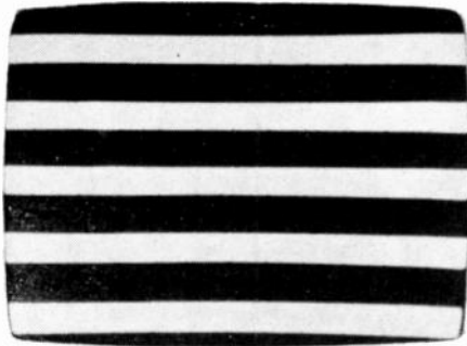
FIG. 5—(above) HORIZONTAL BARS are produced when using signal injector on video amplifier stage.
