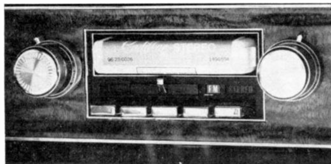
STEREO TAPE is an option on General Motors and other cars. In the dash mounting combines a radio and tape player in the same space originally filled by the radio alone.
