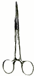
Fig. 15—Hemostats can and are used outside of the operating room. Try these clamping pliers as a handy third hand. The Jonard model M-100-S is shown.
