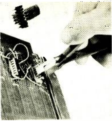
Fig. 18—Getting IC's in and out of sockets can be difficult. But if you use the right tool it's no trouble at all. Techni-Tools' IC Flat-Pack Plier is specially designed to pull IC's without damaging their sensitive pins or placing undue strain on the IC itself.
