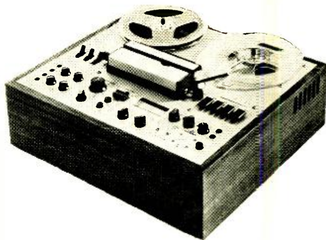
A tape deck using one Dolby frequency band to cut tape hiss is manufactured by KLH.
