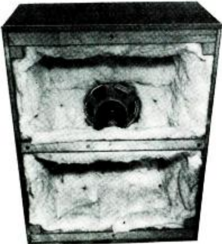
Fig. 3—Inside of speaker cabinet is padded.
