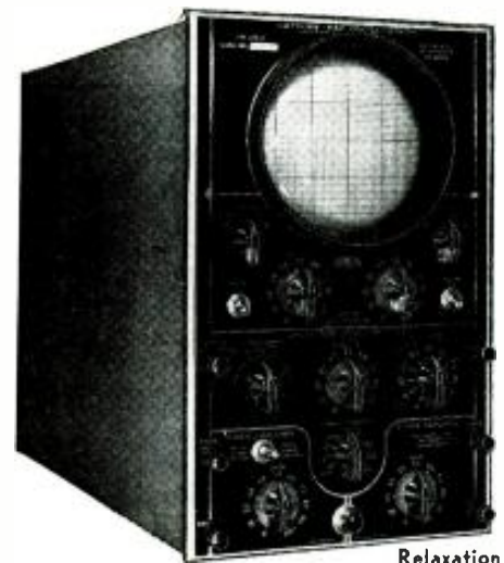
Relaxation oscillator furnishes time base for Dumont oscilloscope.
