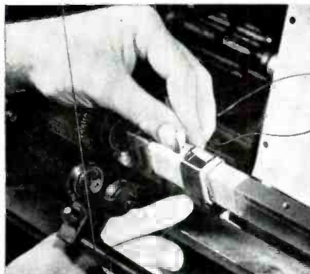
turn through and pull loop ends tight. If winding ends midway, use loop as above, wind a few turns over it and slip end turn through.
