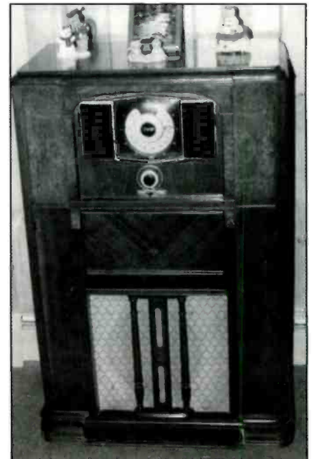
Photo A. This vintage 1942 Zenith "Kenwood" features a shutterdial and pull-out center phonograph.
