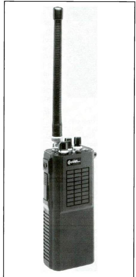
Some low power FM handhelds can operate on two channels, like this one from Fanon Courier, of Tustin, Calif.
