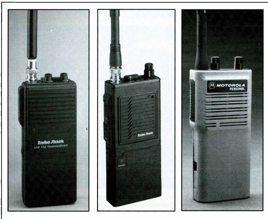
(Left) Radio Shack's BTX-120 is a 1-watt handheld transceiver that comes ready to operate on 154.60 MHz. (Middle) The Radio Shack PRS-100 offers up to seven mile range with 5 watts with two channels in the 462 MHz GMRS band. (Right) Motorola's "Personal 2-Way Radio" operates in the 462 MHz GMRS band.
