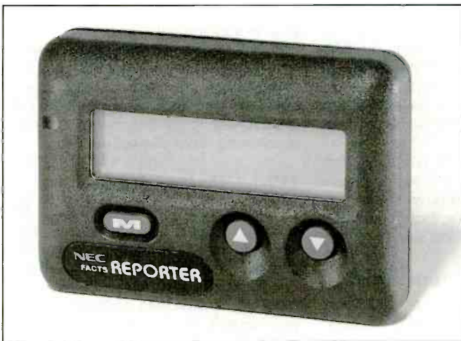
NEC America's alphanumeric pager is called the Facts Reporter. It can store messages for later playback and has eight selectable alerting tones, plus a silent (vibrating) mode.
