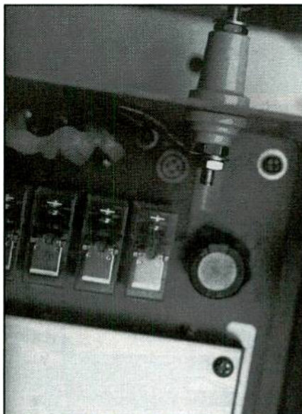
Here is where the ATU feeds through the high voltage R.F. output.
