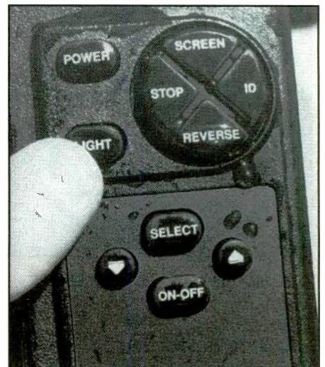
The Hummingbird waterproof keypad keeps water out to 3 feet below water.
