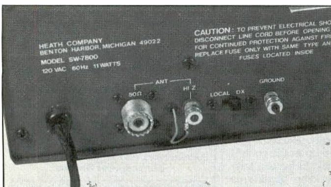
Coaxial (50 ohm) and single-lead (Hi-Z) antenna connectors on rear of shortwave receiver.
