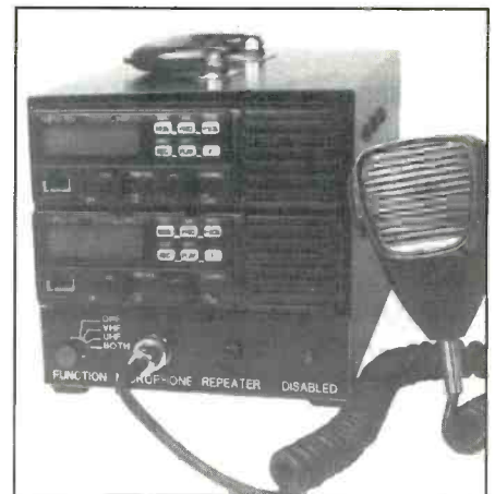
Portable GMRS repeater system for emergency deployment.
