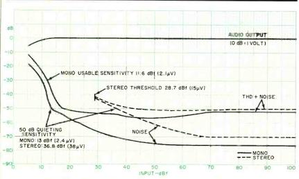
Noise and sensitivity curves for FM section of the SR620CX
