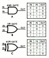
Fig. 1. Three types of gates.
