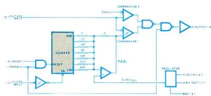
Fig. 1. Internal block diagram of the TL507.
