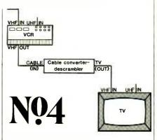
In connection No. 4, the video recorder can record any non-scrambled channel that it can tune-in, and it can program any combination of those channels. The television can tune in any channel, but its remote channel control still doesn't work. You can watch any channel while recording any non-scrambled channel, but you can't record the channels you're paying extra for. If your VCR is not cable-ready, this hookup is particularly limiting.
