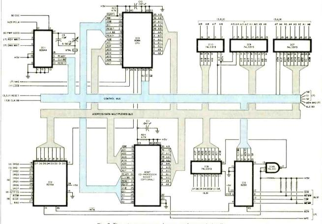
Fig. 2. The microprocessor, buses, and support circuits.
