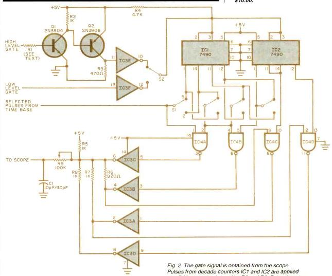
Pulses from decade counters IC1 and IC2 are applied to a D/A converter formed by R5 and R8. Potentiometer R9 and capacitor C1 can be omitted for clock pulses above 1 MHz.
