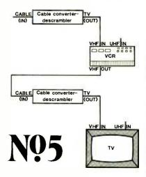
An additional converter/descrambler rented from the cable company and used as shown in connection No. 5 can give you full watch/record versatility and the ability to record scrambled channels. You still won't have full, multi-channel programmability (and you're paying \$3 to \$5 a month for the extra converter). But if you subscribe to a fully addressable system with every channel scrambled, this is the best you can do, although you'll still be doing without remote control.
