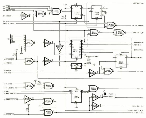
Fig. 7. Motherboard bus arbitration and wait-state generator.
