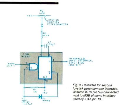
given in the 8080 data sheets.) Therefore, as long as the one-shot is fired, register B is incremented by one count every 18.5 µs. Clearly, then, the value returned in register B is
