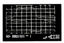
Fig. 3. The aScope/Apple II providing graticule and a pair of traces.
