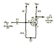
Fig. 2. Basic common-source amplifier.
