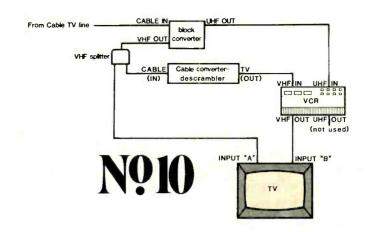
output channel, leaving the remote controls on your video equipment unimpaired. Be sure the distribution splitter will pass uhf (many CATV splitters won't); and don't attempt to use a combined uhf/vhf amplifier in this setup. No uhf/vhf amplifier can handle more than about 7 vhf channels. The thirty or so adjacent channels on your cable system can drive such an amplifier into gross distortion and give you a pretty bum picture.
