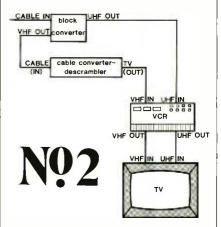
A scrambling system electronically distorts a pay channel in the headend while a set-top converter-descrambler in the subscriber's home descrambles it for viewing. A cable-ready tuner cannot tune a scrambled channel, of course. The number of cable systems using a scrambling system is growing rapidly because the cost of the electronics needed has fallen drastically in the past few years.
