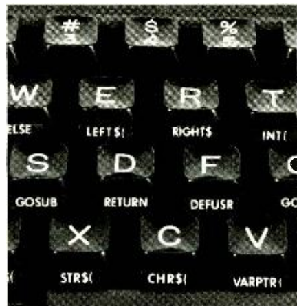
A set of decals can be affixed to keys to indicate command locations.
