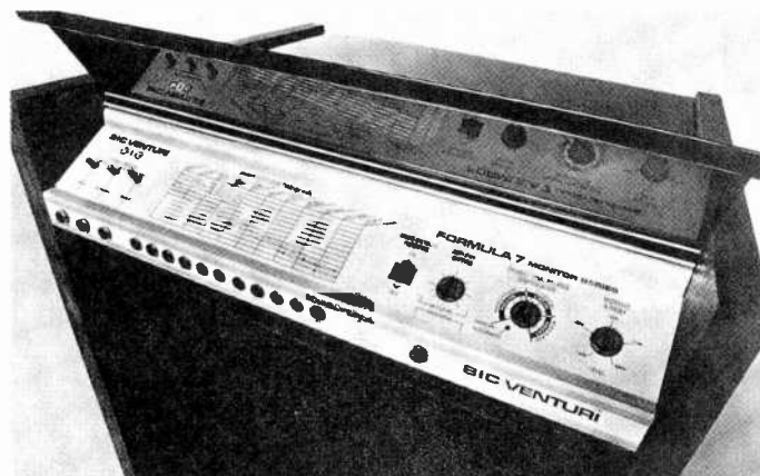
The B.I.C. Formula 7's control panel. The prominent chart facilitates interpretation of the sound-level indicators.
