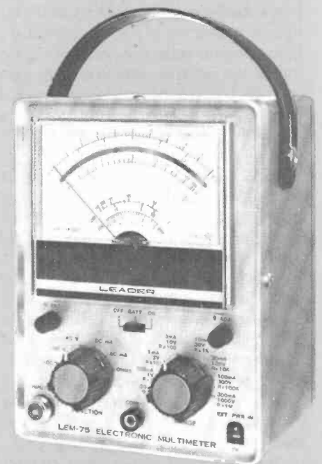
The Leader Model LEM-75, a transistor multimeter, has a temperature scale that is used with an accessory probe.
