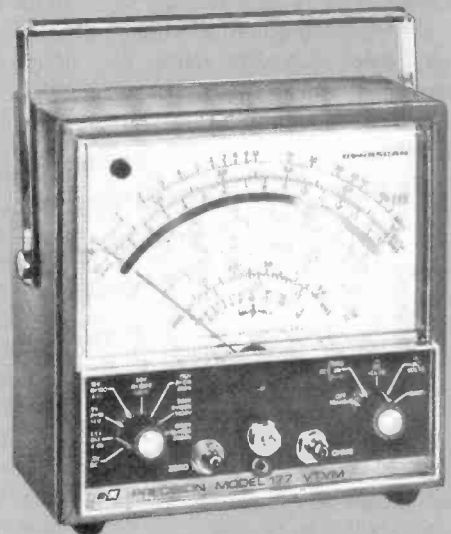
B&K Precision's Model 177 vacuum-tube voltmeter has a large 7" mirrored meter and a special 0.5-V dc scale.
