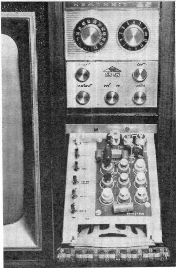
Printed circuit boards and the horizontal output assembly are shown mounted on a vertical swing-out chassis that hinges on the left side of a Magna-Shield ® enclosure designed to isolate the picture tube from external magnetic fields. With the chassis swung open, all test points and terminals are readily accessible for servicing and adjustments.
