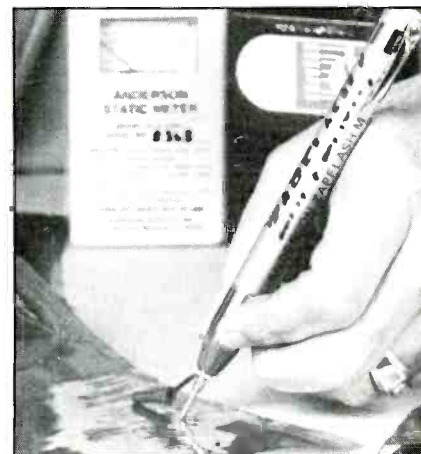
Be cautious with poly bags, which may have exposed carbon or metal on the surface—a shock or ESD hazard.
