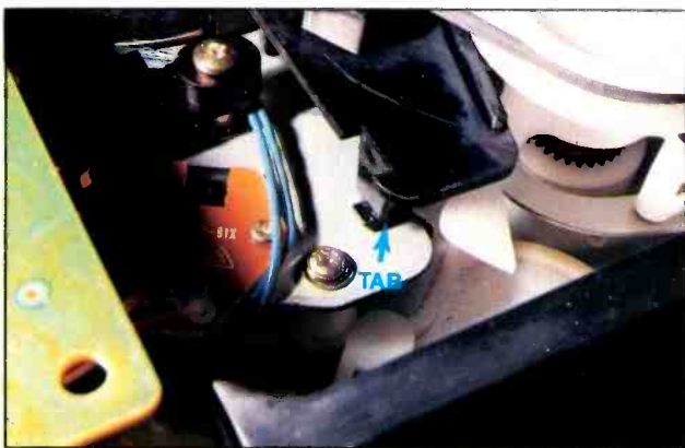
Figure 8. Two tabs secure the plastic bracket to the chassis.
