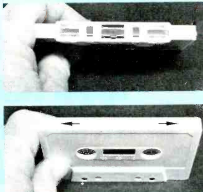
Figure 1 Two views of a standard audiocassette are shown. The housing is made of two identical moldings held together by five screws. (Top) At the left is an opening for the erase head. An opening for the recording/playing head is at the center, and the right-hand opening is for the capstan. Symmetrical construction allows the cassette to be turned over for another recording or playing in the opposite direction, thus doubling the operating time of each cassette. (Bottom) Arrows point to two knock-out-type plastic tabs that determine whether or not the machine can record. This prevents unwanted erasure of recorded material.
