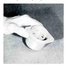
Fig. 1. Tube Socket for High-Voltage Rectifier Employed in Zenith Model X2220R Television Receiver.
