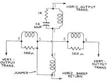
Fig. 8. Schematic of a Yoke in Which Boost Voltage Is Applied to the Vertical-Output Stage by Using Internal Connections in the Yoke.
