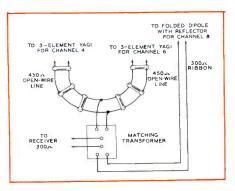
Fig. 3. Clear Beam Antenna System Designed for Indianapolis Area.
