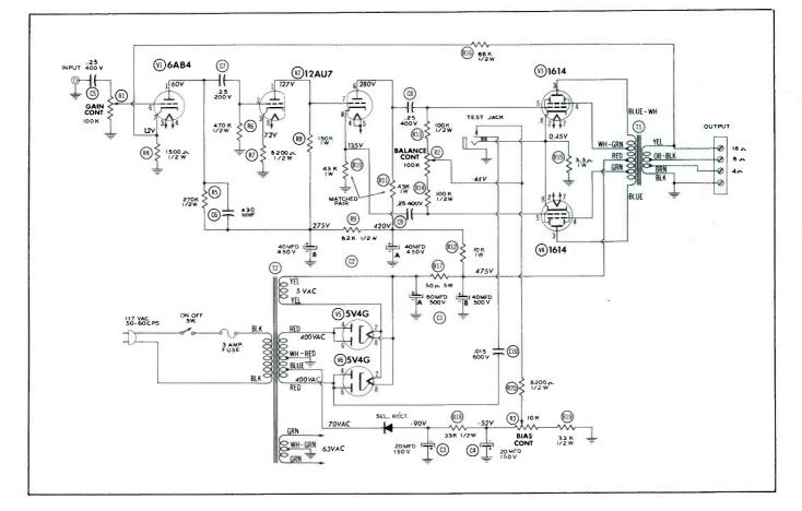
Fig. 4. Schematic of Fairchild Model 260.
