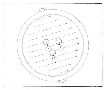
Fig. 9-35. The Field Produced by the Purity Magnet Exerts on Each Beam an Equal Force at Right Angles to the Direction of the Field.
