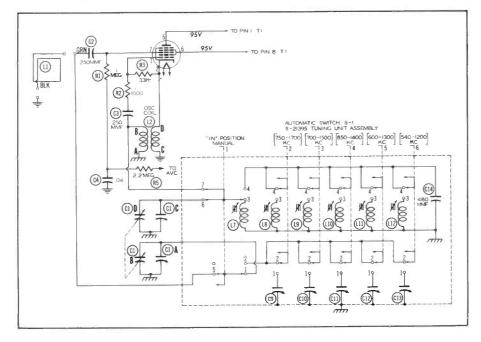
Fig. 8. Tuning Circuits in Zenith Model R512R.
