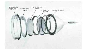
Fig. 9-28. Parts Used in an Early Commercial Color Picture Tube
