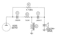
Fig. 6. Schematic diagram of Circuit Used With Electrostatic Speaker in Philco Receiver.
