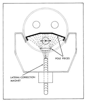
Fig. 9-43. The Field of the Lateral-Correction Magnet Deflects the Blue Beam in a Horizontal Direction.
