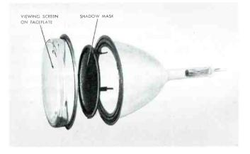
Fig. 9-29. Parts Used in a Later Commercial Color Picture Tube
