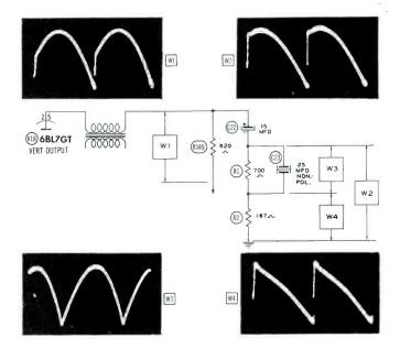
Fig. 9-54. Simplified Schematic of the Dynamic-Convergence Circuit at the Vertical Frequency. (RCA Victor Model 21CT55.)
