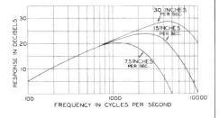
Fig. 3. Curves Showing the Effect of Tape Speed on Frequency Response.
