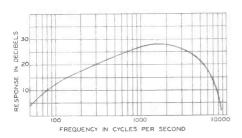
Fig. 1. Typical Response Curve Obtained When Signal Is Recorded and Played Back and There Is No Compensation.
