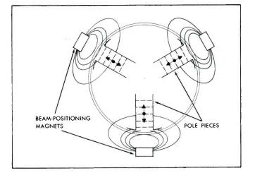
Fig. 9-41. Possible Directions of the Force Exerted Upon Each Beam by the Field of Its Associated Positioning Magnet.
