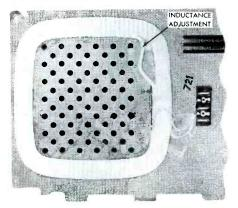
Fig. 1. Loop Antenna with Turns Moved in Order to Change Its Inductance.
