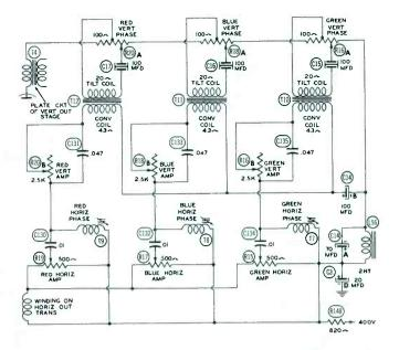
Fig. 9-48. Dynamic-Convergence Circuits Used in the Motorola Model 19CT1.
