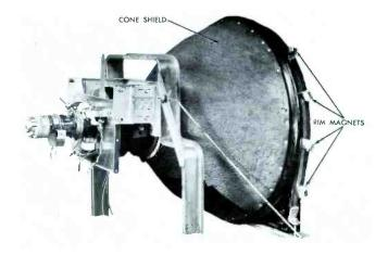
Fig. 9-38. Metal Shield and Rim Magnets Used in Motorola Model 19CT1.
