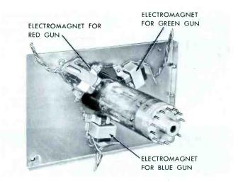
Fig. 9-47. Dynamic-Convergence Electromagnets Used in the Motorola Model 19CT1.
