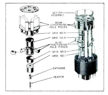
Fig. 9-31. Electron-Gun Assembly Used in a Tube Which Employs the Principle of Magnetic Convergence. (Photograph Courtesy of RCA.)
