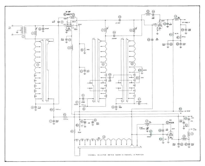
Fig. 12. TV Tuner with Cascode-Coupled RF Amplifier.
