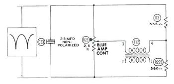
Fig. 9-55. Simplified Schematic of the Circuit Which Supplies the Voltage to the Convergence Coil for the Blue Gun. (RCA Victor Model 21CT55.)
