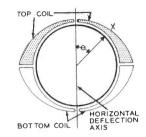
Fig. 3. Distribution of Windings in a Cosine Yoke.
