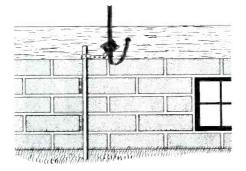
Fig. 2. The Best Position for a Lightning Arrestor Is at the Point Where the Transmission Line Enters the House.
