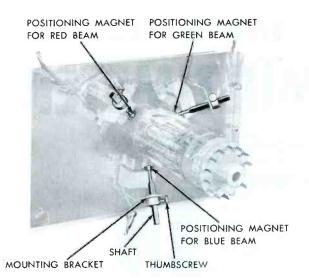
Fig. 9-40. Beam-Positioning Magnets Used in the Motorola Model 19CT1.
