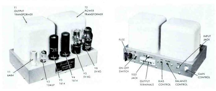
Fig. 1. Front View of Fairchild Model 260 Power Amplifier.
