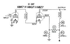
Fig. 11. Simplified Partial Schematic of Cascode-Coupled RF Amplifier.
