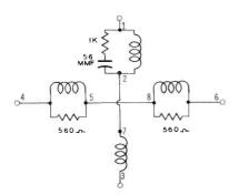
Fig. 7. Schematic of a Typical Deflection Yoke.
