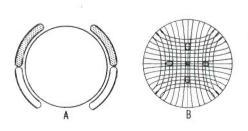
Fig. 2. (A) Cross-Sectional View of One Pair of Deflection Coils. (B) Nonuniform Field Produced by the 50-Degree Deflection Yoke.
