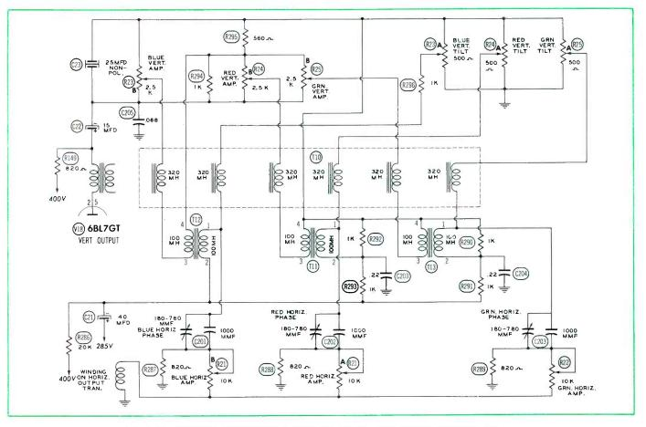
Fig. 9-51. Dynamic-Convergence Circuits Used in the RCA Victor Model 21CT55.
