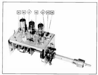
Fig. 1-11B. General Instrument Model 44 Tuner Alignment Points.
