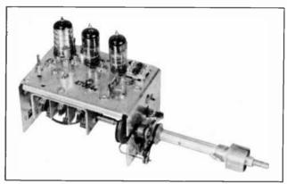
Fig. 1-11A. General Instrument Model 44 TV Tuner.
