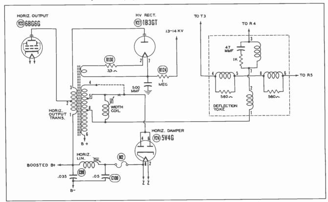
Fig. 6. Schematic of Horizontal Sweep Circuit after Conversion.
