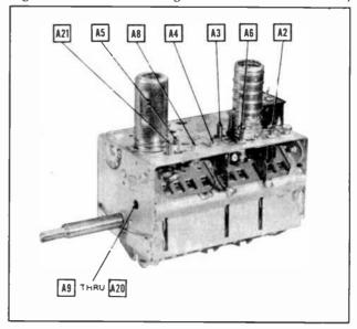
Fig. 1-12C. Hallicrafters Printed Circuit Tuner Alignment Points.
