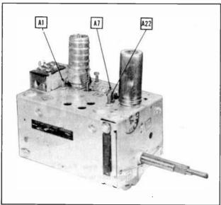
Fig. 1-12B. Hallicrafters Printed Circuit Tuner Alignment Points.
