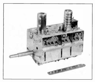
Fig. 1-12A. Hallicrafters Printed Circuit Tuner.
