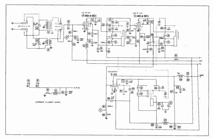
Fig. 1-11K. Schematic of General Instrument Model 44 TV Tuner.
