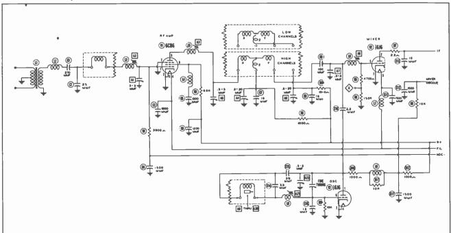
Fig. 1-12G. Schematic of Hallicrafters Printed Circuit Tuner.
