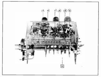
Fig. 1-11C. General Instrument Model 44 Tuned Circuit Coils.
