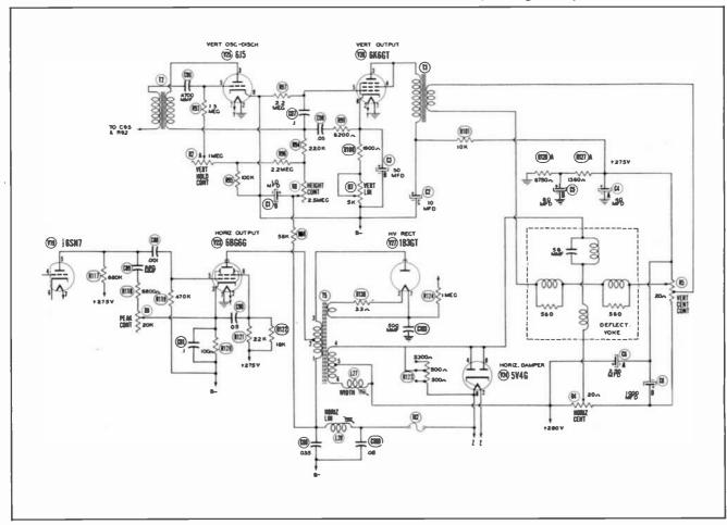
Fig. 2. Schematic of Horizontal and Vertical Sweep Circuits before Conversion.
