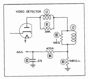
Figure 1. Conventional AGC Circuit.
