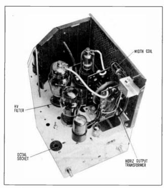
Fig. 7. HV Compartment Showing New Components.
