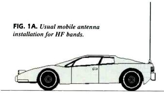
horizon. Increasing the height of the antenna increases the line-of-sight distance. Of course, if you can possibly rig up a repeater, then that's even better.
