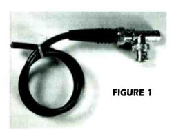
critical and it is determined by both the frequency you want to reject and something called the "velocity factor" of the coax cable.
