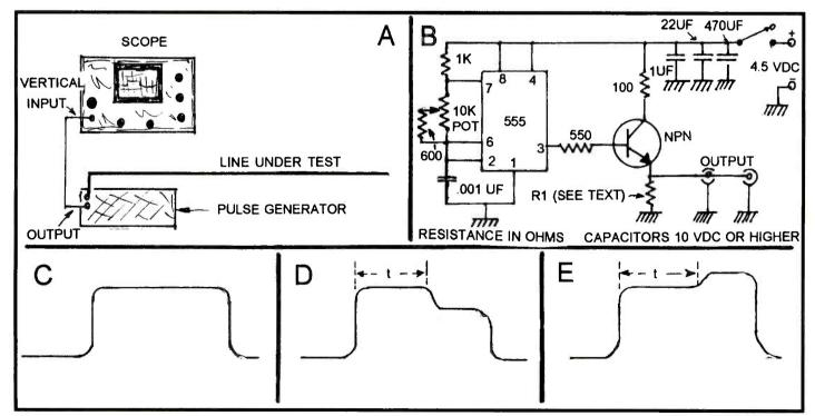
**FIGURE 1.** A basic TDR system (A), pulse generator diagram (B), typical pulse shape (C), shape of pulse combined with reflections from short-circuited cable (D), shape of pulse combined with reflections from open-ended cable (E)
