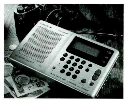
years. It covers longwave, the AM band to 1710 kHz, and the usual FM band—in stereo through headphones (not supplied). Shortwave is completely covered, continuously from 1.72-30.0 MHz. There are the same two major drawbacks, as before: no main tuning knob and no synchronous selectable sideband.
