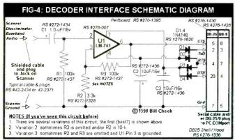
spect to the polarity of the capacitors and diodes. The decoder interface should be as close to the PC as possible to minimize stray RF emissions from the serial port. (That's why putting the interface inside a DB25 connector shell is best.) The cable from the interface to the scanner's baseband audio jack must be shielded. The shield connects to ground of the decoder interface at the one end and to scanner ground at the other end.
