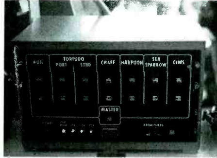
Weapons station. Note the simplicity: two push buttons/indicators for each system. The top one indicates the status as either Enable or Veto. The bottom one is a Veto push-button, and then there is a Master Veto.
