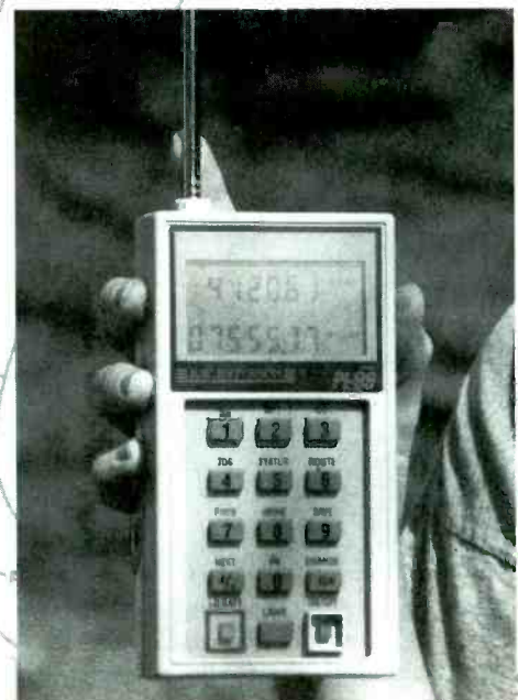
A close-up of the Ray Jefferson, PL-99 LORAN-C receiver. Notice the different options for display: long/lat, time differences, route, waypoints, etc.
