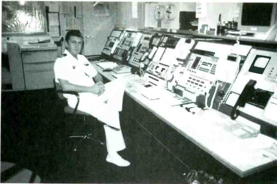
Gone are the days of messages being sent by Morse code. Here, Chief Radio Officer Terje Johnsen sits in the radio room in front of the console housing some of the ship's communications equipment including a 1 kW HF rig.
