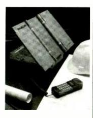
Bob Grove set up the Magellan MicroCom-M satellite telephone on an old picnic bench in the middle of the North Carolina woods. The thing is remarkably easy to get going. You turn the unit on, unfold the two panels that act as the antenna, and point it at the nearest satellite. (You know when you're on target by watching the LED light bar.) All that's left to do is to pick up the handset and dial!
