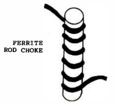
Methods for using ferrite toroids and rods for RFI suppression. These chokes should be located as near to the equipment chassis as possible for best results. Amidon FT-240-43 or FT-240-43 toroids (see text) are suitable for winding toroid chokes Ferrite rods are scarce on today's market, and they are quite expensive. The ferrite bars and rods on which AM radio loop antennas are wound may be used for choke forms. They have a permeability of approximately 125 (no. 61 material).
