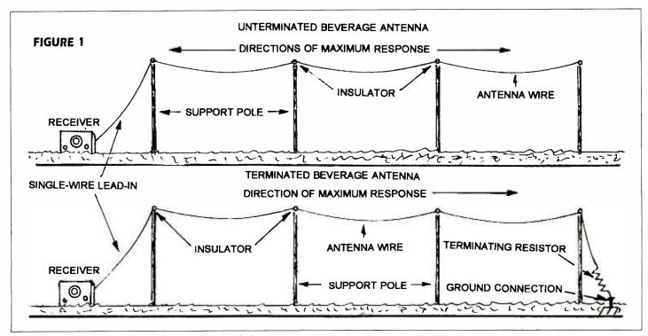
Two configurations of the basic Beverage-antenna design.
