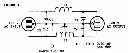
Circuit for a brute-force ac line filter. The coils are wound on broom handle sections, dowel rod or PVC tubing (see text). Capacitors are 0.01-µF, 630-VDC units (see note 1). One male and one female ac receptacle are required for this filter. It must be enclosed in protective box for reasons of personal safety.
