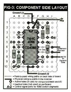
4 show how to build the simple circuit on a piece of perfboard. Connection and hookup are not critical. The primary consideration is where to make the connections. In all cases, the path between the hysteresis resistor and pin 14 must be cut and the "contacts" of the 4066 switch wired to each side of the "cut."
