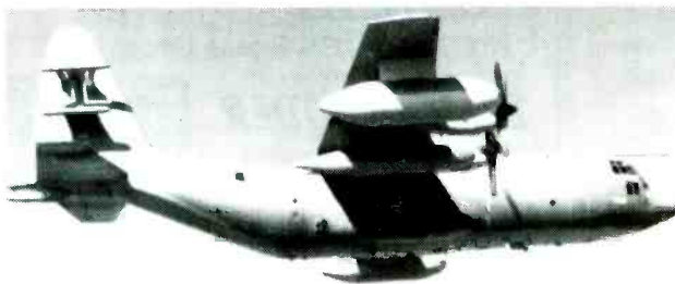
FIGURE 1: Although this Rivet Rider C-130 Hercules “psychological operations aircraft” is bristling with exotic antennas, some are not so obvious, being hidden in pods or even under the skin of the aircraft. The lower profile antennas are especially desirable in supersonic aircraft, where even an antenna covered by a pod creates wind resistance. (Courtesy Lockheed/Dept of Defense)
