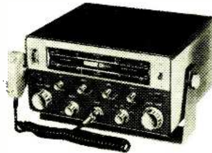
The Heathkit Shawnee or Pawnee will provide good-sounding AM or CW operation on VHF at bargain prices.
