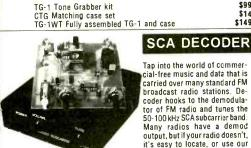
cial-free music and data that is carried over many standard FM broadcast radio stations. Decoder hooks to the demodula-tor of FM radio and tunes the 50-100 kHz SCA subcarrier band. Many radios have a demod output, but if your radio doesn't, it's easy to locate, or use our FR-1 FM receiver kit which is a
