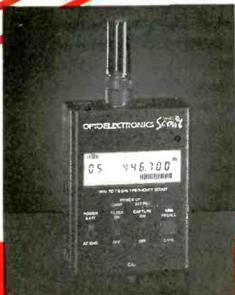
Reaction tunes VHF/UHF receivers equipped with CI-V serial communications interface.
