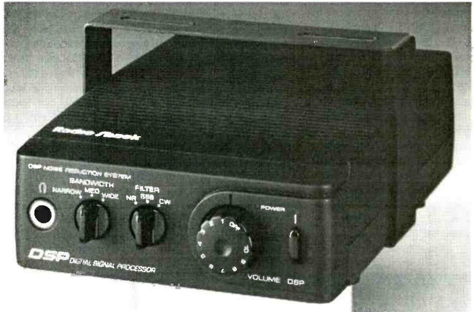
be selected from 300-3000 Hz wide (no filtering) to 597-903 Hz narrow CW.
