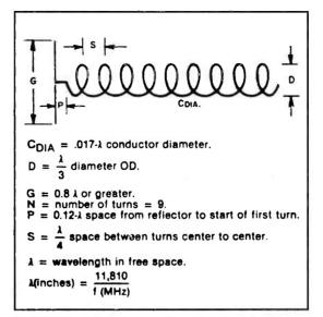
FIGURE 1: Design equations for circularly polarized antennas (courtesy of American Radio Relay League).
