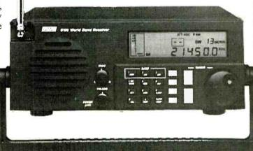
For example, although SW8 comes with a number of useful features, it lacks some of the signal-enhancing features of the R8. For example, there's no passband offset or notch filter.
