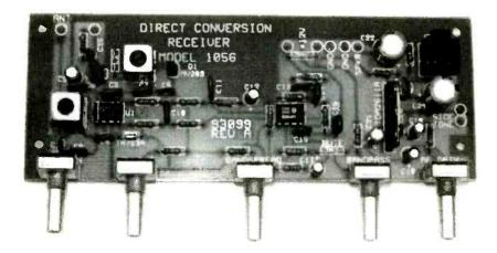
Ten-Tec 1056 CW-SSB receiver kit in its bare bones configuration.
