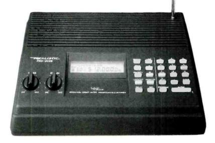
For those individuals who do not require a scanner with 800 MHz capability, the Realistic® PRO-2028 offers 50 memory channels in ten five-channel banks and a frequency coverage of 29-54, 108-174 and 406-512 MHz. Additionally, five temporary ("scratchpad") channels can store frequencies discovered during the search routine.
