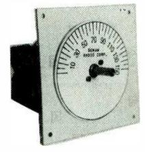
**Figure 1:** Photograph of a home-made tuning dial. Single-sided PC board stock is used for the square and circular plates. This assembly mounts behind a clear plastic window that is glued to the inner edges of a cutout on the front panel. The window has a vertical line that has been scribed in the plastic and filled with India ink to provide a reference line for the dial numbers.
