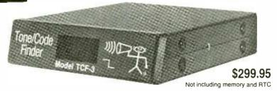
The Tone/Code Finder is composed of a high speed display unit coupled to your receiver. IT'S PURPOSE IS TO INSTANTLY FIND AND DISPLAY ALL CTCSS AND DIGITAL CODES, INCLUDING SPLIT CHANNEL AND INVERTING CODES.
