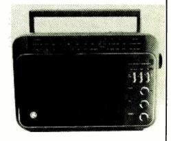
tunes from 530 to 1700 kHz, allowing reception of TIS (travelers information stations) as well as the newly expanded mediumwave broadcast band.
