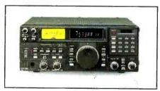
The IC-R71A is a shortwave listener's delight. Its **32 tunable memories** store frequency and mode information, and they are single-button reprogrammable **independent of VFO A or VFO B's operations!** Dual width, an adjustable noise blanker, panel selectable RF preamp, and selectable AGC combined with **four scan modes** and all-mode squelch further enhance the IC-R71A's HF reception!
