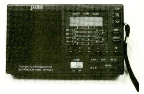
After all this, the remaining characteristics seem relatively palatable. Selectivity is downright poor—Chinese radio designers apparently haven't yet caught on that good adjacent-channel rejection has been a key variable in shortwave receiver design since the Truman era. But sensitivity is at least okay for basic shortwave listening; ditto audio quality.
