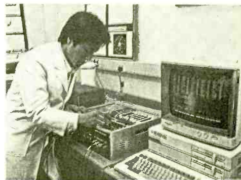
A KSRI Time and Frequency Lab technician works on the joint Japanese-Korean developed GPS interface prototype.
