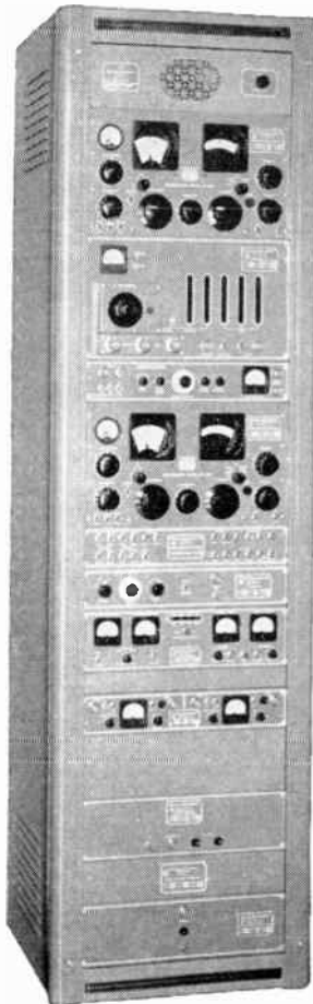
TYPICAL RECEIVER TERMINAL for TWINPLEX OPERATION
