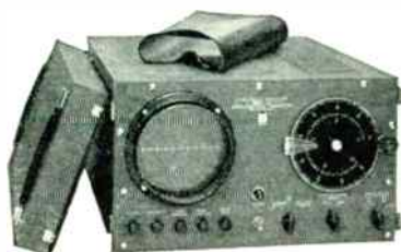
Sierra 124A Line Fault Analyzer
