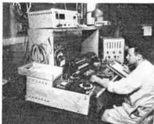
Reliability testing being performed using automatic check out panels.
