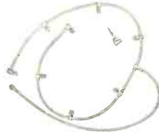
THERMOCOUPLE HARNESS: Flexible, completely sealed and suitable for continuous operation in ambient temperatures of -65°F to 1500°F. Thermocouples are singly detachable and the sealed harness eliminates any chance of trouble from altitude, moisture or other contaminants.
