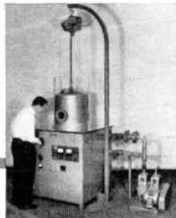
Belljar and tank vacuum metallizers, diameters 12" to 66", for depositing thin films to precisely controlled thicknesses of from one molecule to several mils.
