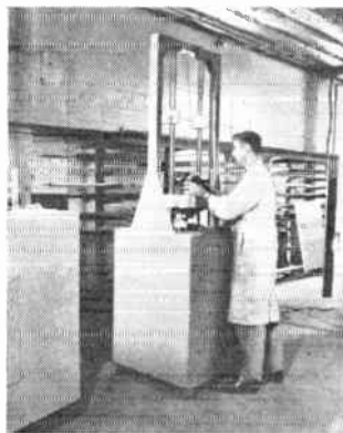
Sawtooth shock test being performed on a Shock Test Machine developed by Associated.
