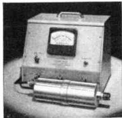
Model 520 Alphatron® Ionization Gauge. Range 1000 — 0.0001 mm Hg.
