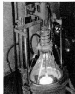
Low-cost standard furnace for growing single crystals of silicon, germanium, and intermetallic compounds.
