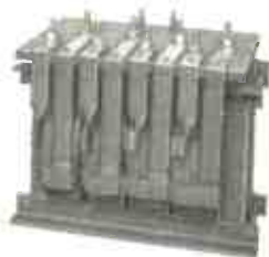
Filament Transformer, 400 cycles with 4 secondaries, 10 volts, 100 Amperes. Each secondary can be mounted in parallel series or series parallel.
