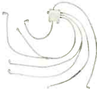
CONTROL HARNESS: This configuration, encased and sealed in metal braid and complete with junction box, can safely withstand the adverse effects of engine environment such as heat, vibration, and oils.
