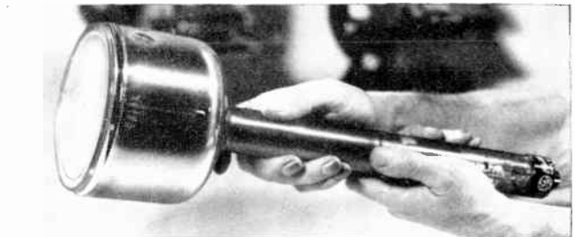
Thoroughly researched and job-tailored, Z-4448 transparent phosphor tube offers ultra-high resolution for specialized photographic applications.
