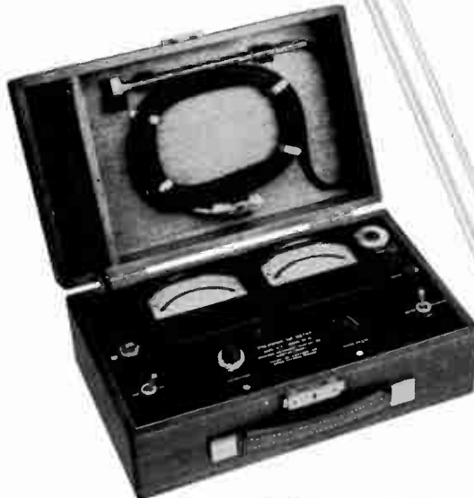
Hastings Model B Air Meter for measurements of greatest precision. Velocity ranges: 0-400 fpm; 400 to 6,000 fpm. Meter type continuous calibration check. Knife edge, paral- lax free indicator.
