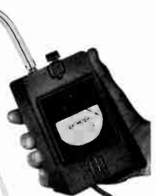
Hastings Model G Air-Meter. Small hand type instru- ment. Velocity range: 0-6000 fpm; Weight: 26 ounces.
