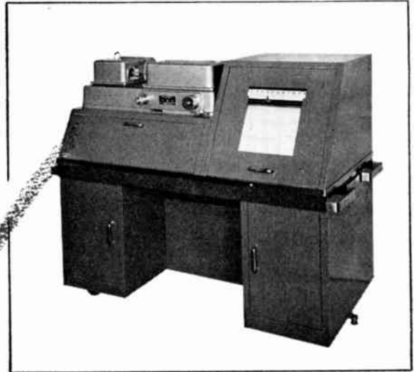
Above: Perkin-Elmer infrared spectrometer —in its Karp-built cabinet, below.
