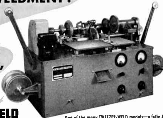
One of the many TWEEZER-WELD models—a fully Automatic Double Tabbing Machine for miniature tube cathodes.
