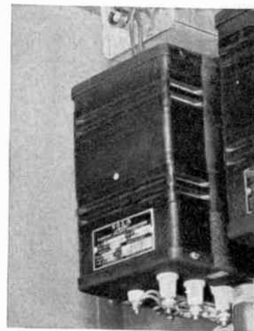
STATIC-MAGNETIC REGULATION. Standard Sola stabilizers are available in capacities from 15va to 10kva, and with a variety of common power line and filament voltages. Special designs can be produced for quantity orders.
