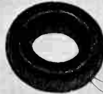
1-1/8" O.D. x 3/4" I.D. Wire—44 AWG Winding Speed—800 rpm
