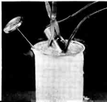
5. At -55 degrees centigrade, the subminiature G-E metal-clad capacitor with Permafil dielectric shows less than 7 percent loss in capacitance.
