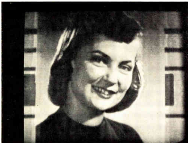
Actual scan using RL512 array. Scan rate, 2 MHz; Resolution, 6 mils; 4 bit A/D conversion provides 16 gray levels. Photo is courtesy of Recognition Equipment, Incorporated. (see Note)
