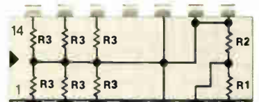
899-40 DIP network provides six line terminators and the threshold setting divider for the Intel 3208A sense amplifier. Price (1,000-4,999) $1.35
