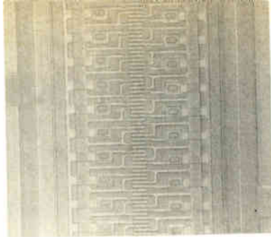
2. By the line. Linear charge-coupled imagers for both printed and pictorial information have been built. Device on left is a three-phase 500-element linear array. On the right is a 1,500-element array which is capable of far greater resolution.
