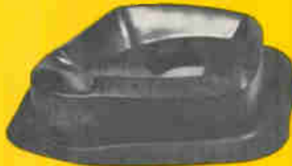
Cold Rolled Steel; 22" diameter, .024" blank One draw • 7,000 psi
