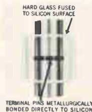
TERMINAL PINS METALLURGICALLY BONDED DIRECTLY TO SILICON
