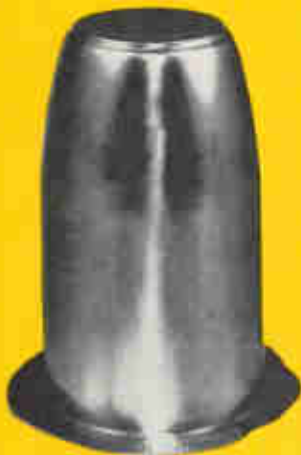
Brass 70-30; 12" diameter, .35" blank One draw • 12,000 psi
