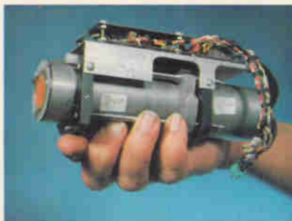
Up tight. Camera-head optics and electronics, above, have been squeezed into a small package. At left is the lead-oxide pickup tube with deflection yoke and preamplifier.
