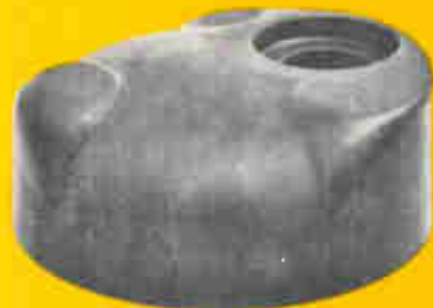
Stainless Steel 302; 7" diameter, .020" blank One draw • 10,000 psi
