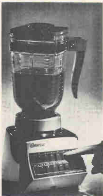
Kitchen aid. Food blender, designed with Motorola integrated circuits, will soon be made available by John Oster Manufacturing. The design eliminates push buttons and switches. Speed selection is made by touching insulated capacitance plates.
