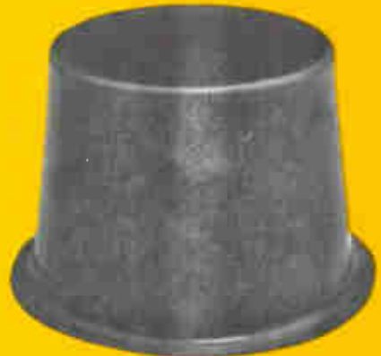
Stainless Steel 304 12" diameter, .030" blank Two draws • 14,000 psi
