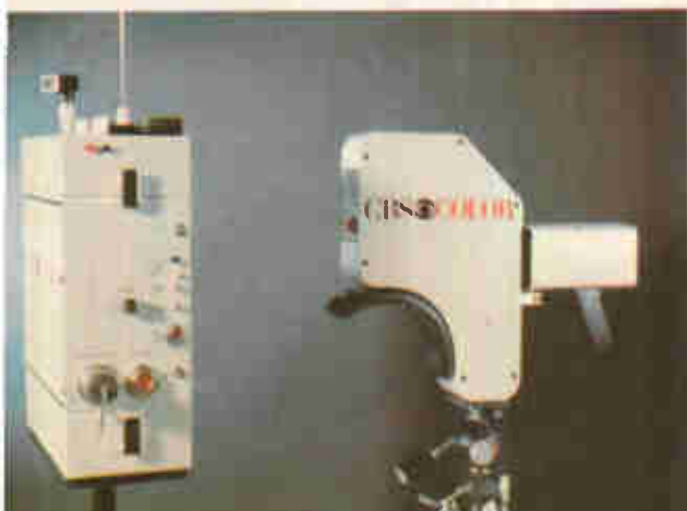
The Minicam. Essentially a low-power tv transmitter, the system sends an NTSC signal to remote base station.
