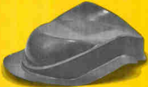
Aluminum 5257-0; 12" diameter, .035" blank One draw • 5,000 psi
