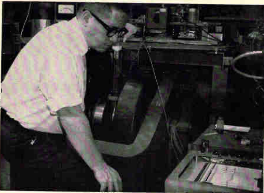
Scientist watches readout of electron-spin resonance device (to his left) that is testing a sample of human tissue for cancer. The device detects malignancy because of the peculiar way the diseased tissue reacts in an intensive magnetic field.
