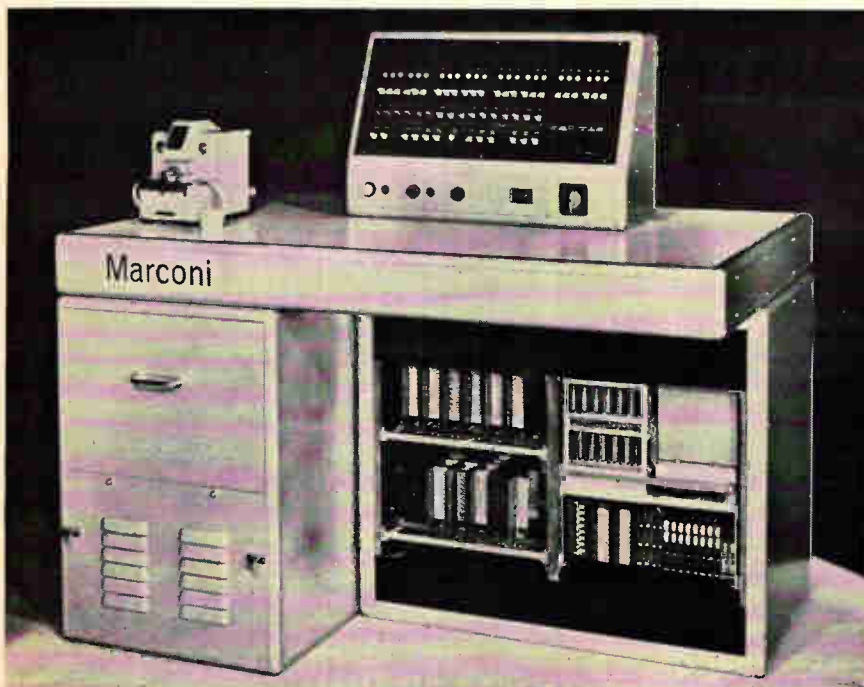
Achievement of British microelectronics is Marconi Co.'s desk-size Myriad computer measuring 6 by 3 by 2½ feet. It has 4,096-word capacity, can add and subtract in 2.5 microseconds and multiply in 10 microseconds. Maximum time before failure is said to be 30,000 hours, compared with 3,500 hours for most conventional models. First model has been sold to Royal Radar Establishment at Malvern.
