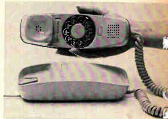
Dial-in-the-handset telephone introduced by Bell System. Printed circuit fits into curved handset, which weighs only two ounces more than a conventional handset but contains the dial, wires, other gear.
