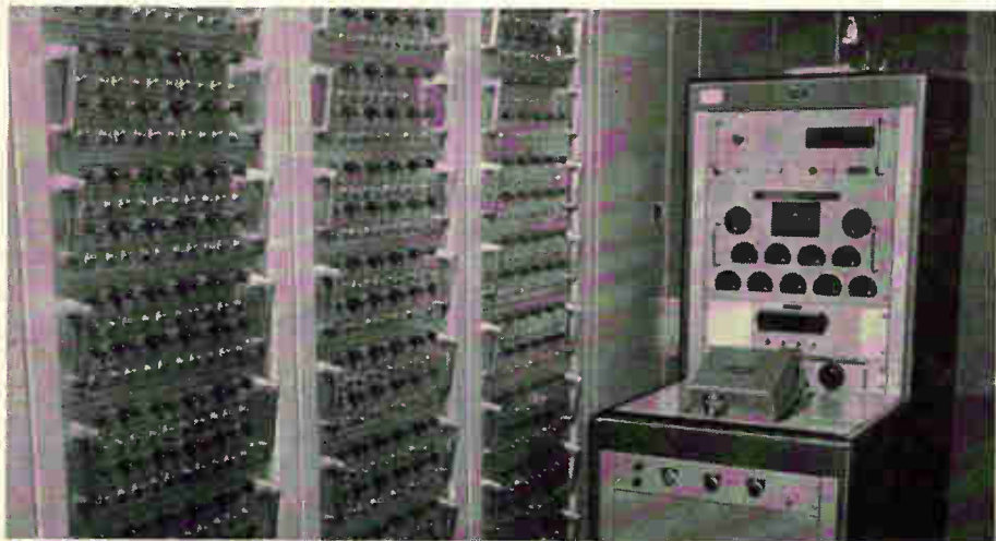
In order to accommodate the 10,000-hour failure-rate level determination load life test (shown above) as well as the other special tests required by MIL-R-39008, Speer recently added 28,000 square feet of quality control and inspection facilities to its Bradford, Pennsylvania, resistor plant.
