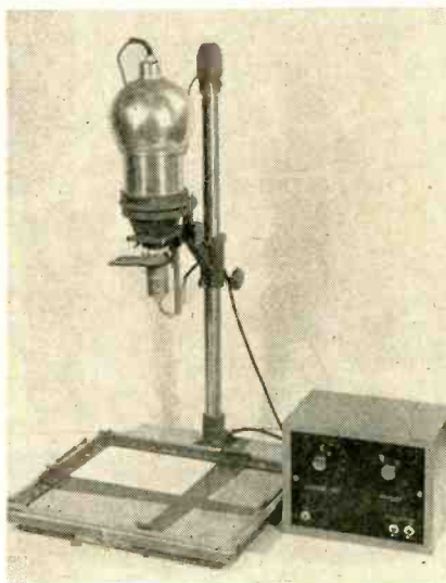
Print timer is shown beside the enlarger with the filter-switching motor mounted in place of the red filter normally supplied with the enlarger. The two color filters are mounted on an aluminum plate attached to the motor shaft. Shock mounts prevent jarring of enlarger when switching filters to change contrast
