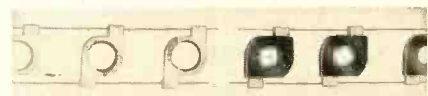
Cast zinc cores, bare at left and insulated with black nylon at right, are shown before spring wire brushes are cut and bent
