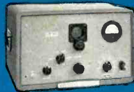
650A —highly stable, wide band; 10 cps to 10 MC. For audio, supersonic, video, rf measurements. Output 15 mw/3 volts. Frequency response flat \pm 1 db. $490.00
