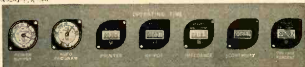
The illustration shows how the operating time of various sections of an electronic console can be monitored.
