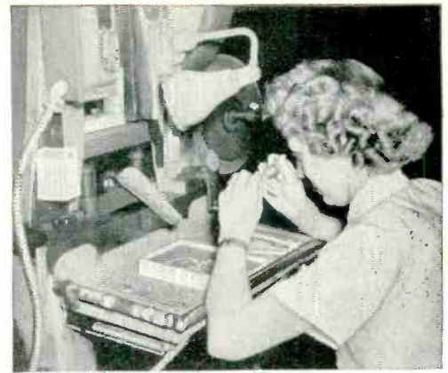
Part of Inspection Procedure on Lockseam Nickel Cathodes as they come off the production machine. Each cathode must undergo many rigid tests before being approved.
