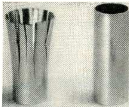
Both tubes were "sunk" or drawn without a plug to induce stresses. Tube (left) was then annealed at the base only and tube (right) was annealed its entire length. After testing in mercurous nitrate solution, cracking revealed the presence of severe internal stresses that were present in the unannealed portion of the tube.
