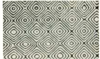
FIG. 11—Square-net domain pattern of single barium titanate crystal, visible because crystal is transparent
