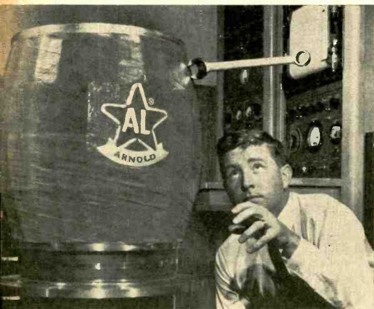
Barrel-Shaped Magnet. (Above) A large, barrel-shaped magnet assembly made of an improved magnetic alloy, Alnico 8, has been developed for use with super-power klystron tubes. The magnet, made by Arnold Engineering, is 27½" high and weighs ½ ton. Previous assemblies made for the microwave industry weighed from 1200 to 1400 lbs. but used a lower-energy Alnico 8. The new alloy, like others in the same family, is heat-treated in a magnetic field to develop its high coercive force and energy product. The main axial klystron cavity magnetic field is more than 1050 gauss with a very low cross field.
