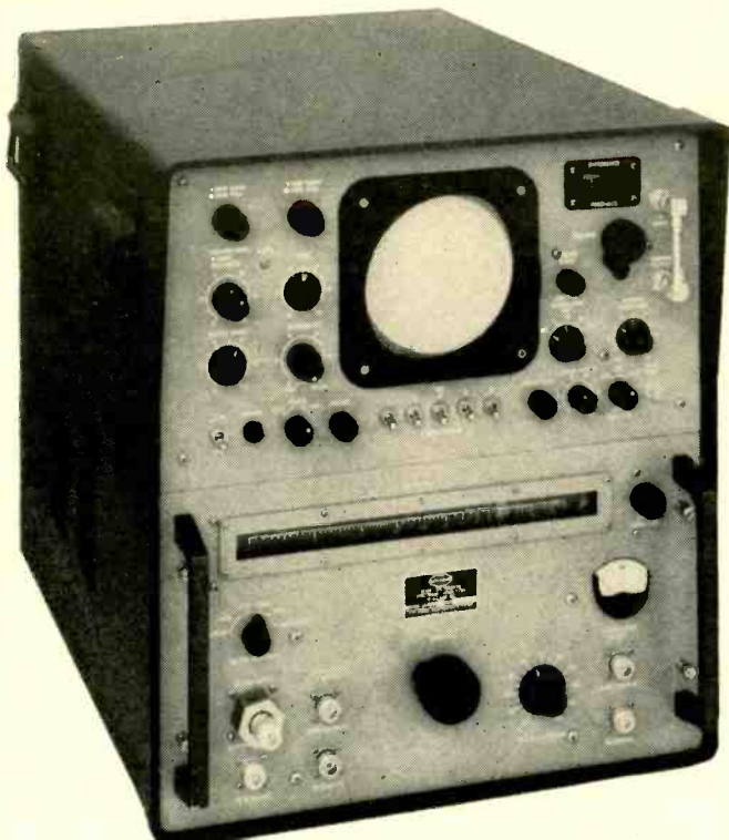
This extended-range microwave spectrum analyzer is Polarad's Model SA-84WA. It covers the region from 10 mc. to just over 63 gigacycles in 10 bands with a single tuning unit. Variable frequency marker is built in, as is 0.01% crystal marker.
