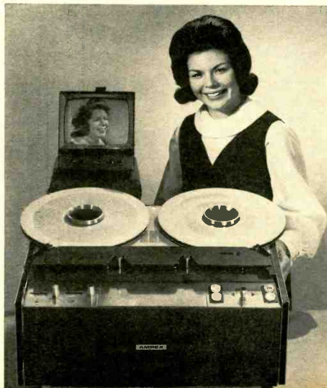
Low-Cost CCTV Video Tape Recorder. (Below) A new compact TV recorder designed for closed-circuit systems is being marketed by Ampex at about half the cost of previously available comparable equipment. The recorder is priced just under $4000. The unit uses a single stationary video head that lays a longitudinal track along the length of the ¼" tape, which moves at 100 ips. A 12½" reel of 12,600 feet of special ½-mil video tape will provide a playing time of 25 minutes. The tape direction then reverses and another 25 minutes of playing are available. A reel of tape sells for $58. The video bandwidth of the new recorder is 250 cps to 1.5 mc. (at -3 db).
