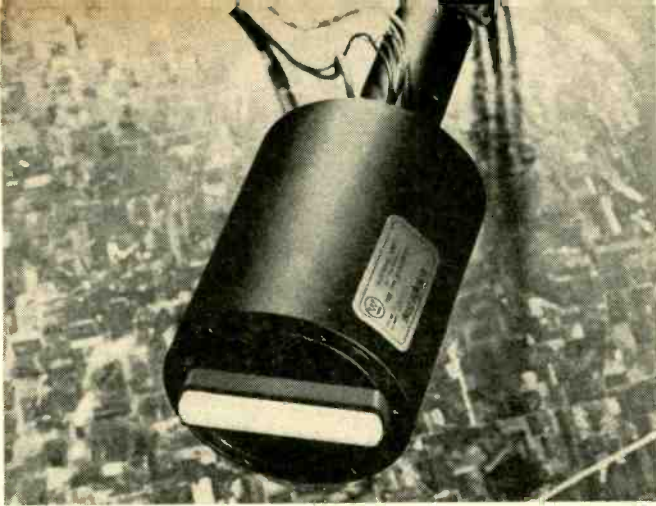
This special CRT puts single-line scans from high-resolution radar directly onto film—producing permanent records of near-photographic quality. The raised portion of the tube face contains the fiber-optic element that touches the photographic film.
