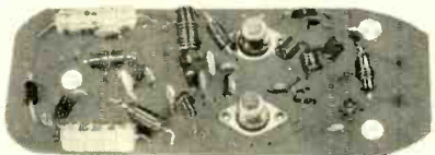
UNRETOUCHED PHOTOS OF PRINTED CIRCUIT AND POTTED COMPONENT SIDES OF TELE-AMP AMPLIFIER BOARD AFTER 204-HOUR WEATHER-TORTURE TESTS
